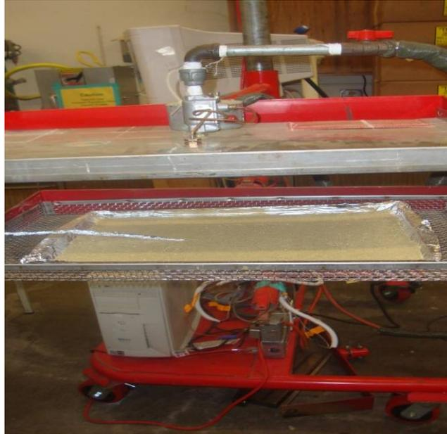
Fig. 2. Infrared treatment of rice bran.
