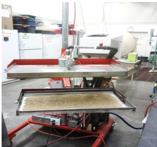
Fig. 1. Infrared treatment of rough rice.
