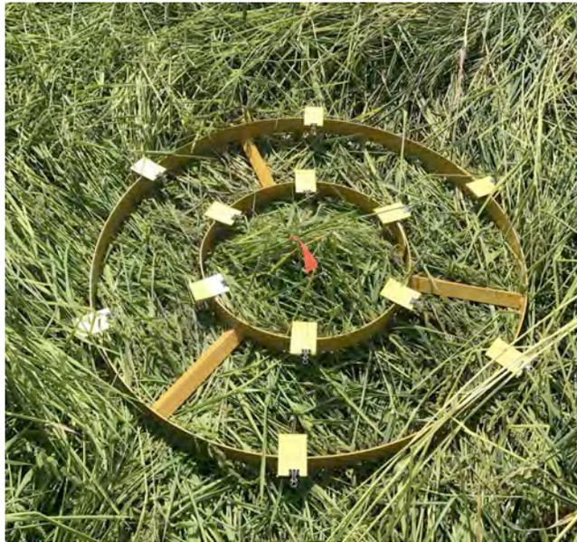
Fig. 4. Bullseye ring with water-sensitive paper positioned at mapped target.
