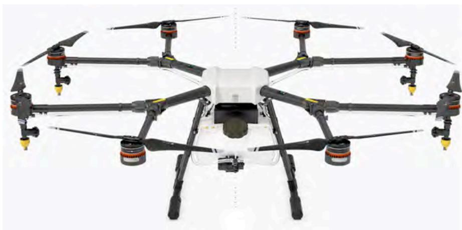
Fig. 1. The DJI Agras MG-1 Multi-rotor helicopter for agricultural spraying (manufacturer’s graphic).
