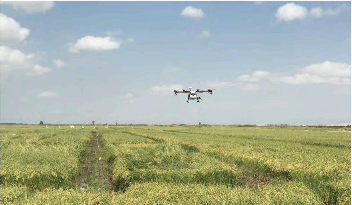
Fig. 5. Aircraft positioned by reference to GPS target and hovering to make spray spot treatment.
