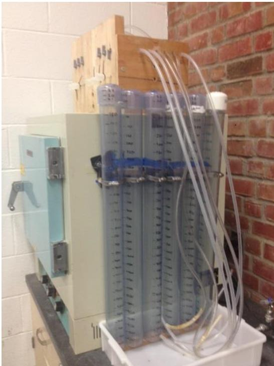
Figure 6. Equipment to measure volume of biogas generated with inverted columns of water.
