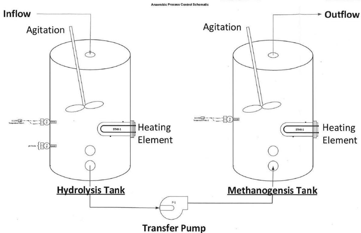
Figure 9. Design of anaerobic digestion tank of a100 gallons.
