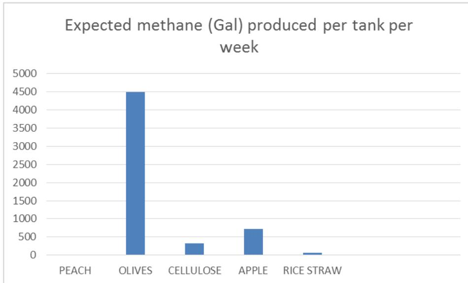
Figure 8. Expected methane generation in gallons in 100-gallon AD reactor
