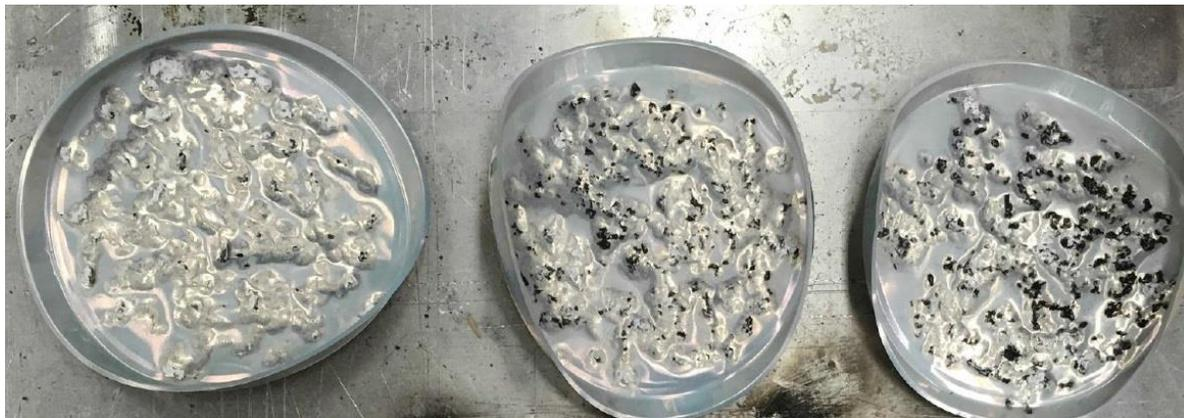
Figure 3. *Burn-off test results for percentage of carbon*
