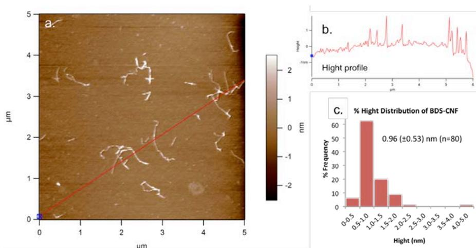
Figure 4: AFM image of BDS-CNF generated from the optimized reaction. (a) 0.0003 vol% BDS-CNF in aqueous solution. (b) Height profile. (c) % Width distribution of BDS-CNF with the average of 0.96 (±0.53) nm.
