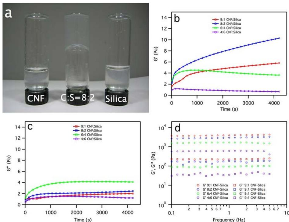
Figure 3. (a) Photo of 0.6 wt% of CNF, silica and 8:2 CNF:silica aged for 48 h; viscoelastic properties of CNF/silica hydrogel. (b)  $G'$  and (c)  $G''$  of hydrogels during time sweep; (d)  $G'$  and  $G''$  of hydrogels aged for 48 h aging and cured in 0.2 N HCl during frequency sweep.
