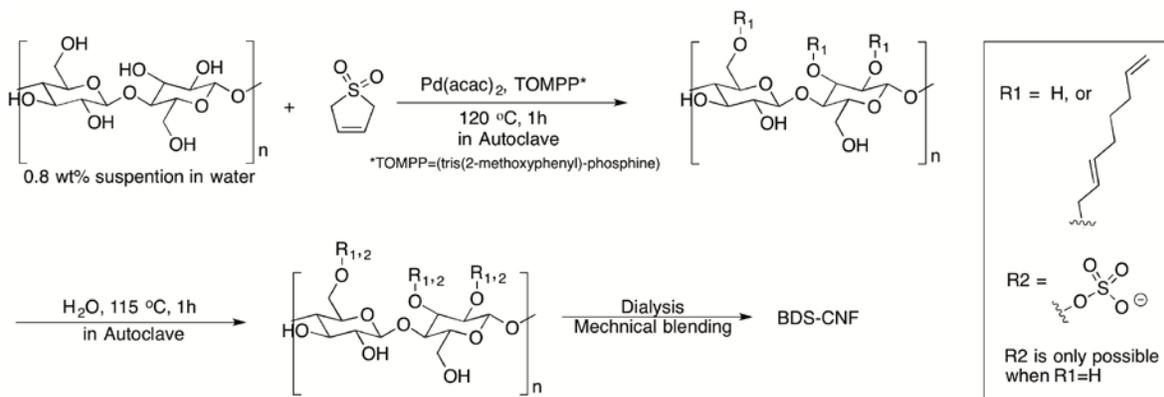
**Scheme 1:** The reaction route for telomerization and acid hydrolysis to generate hydrophobic cellulose nanofibrils (BDS-CNF).
