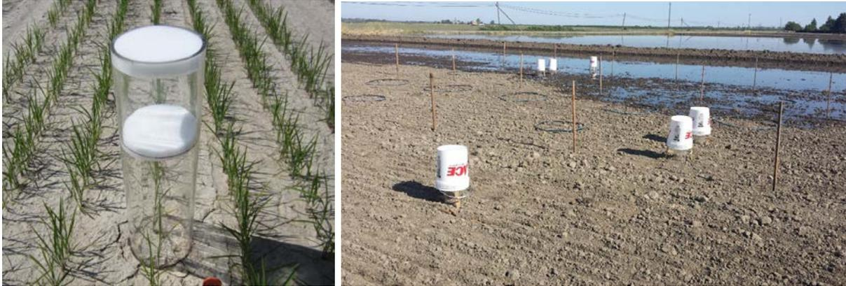
Figure 4-5. Pictures of the chambers used to measure  $\text{NH}_3$  volatilization in the field. The foam contains phosphoric acid which captures the  $\text{NH}_3$ .
