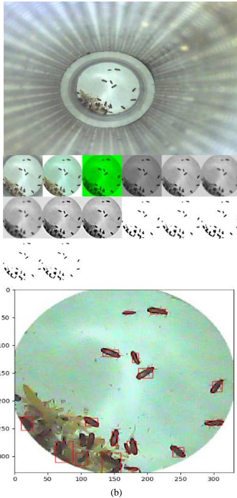
Fig. 13. Image processing algorithm stages and final image processing output.
