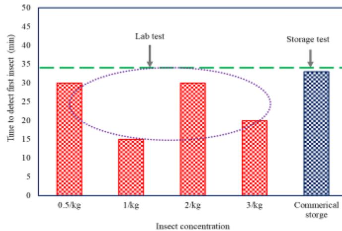
Fig. 16. Time to detect the emergence of the first insect during the lab and commercial storage tests.
