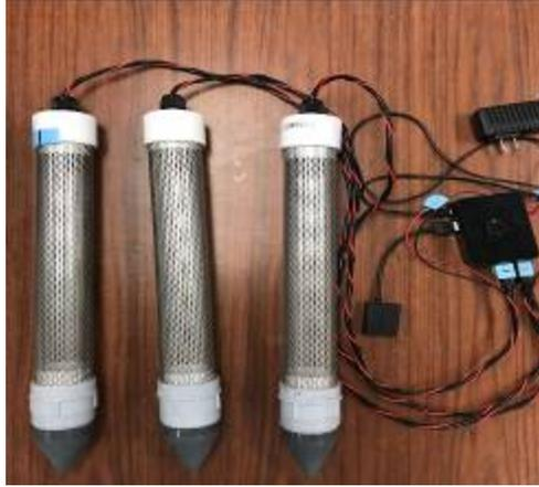
Fig. 3. Designed traps with installed LEDs, camera, and raspberry Pi.
