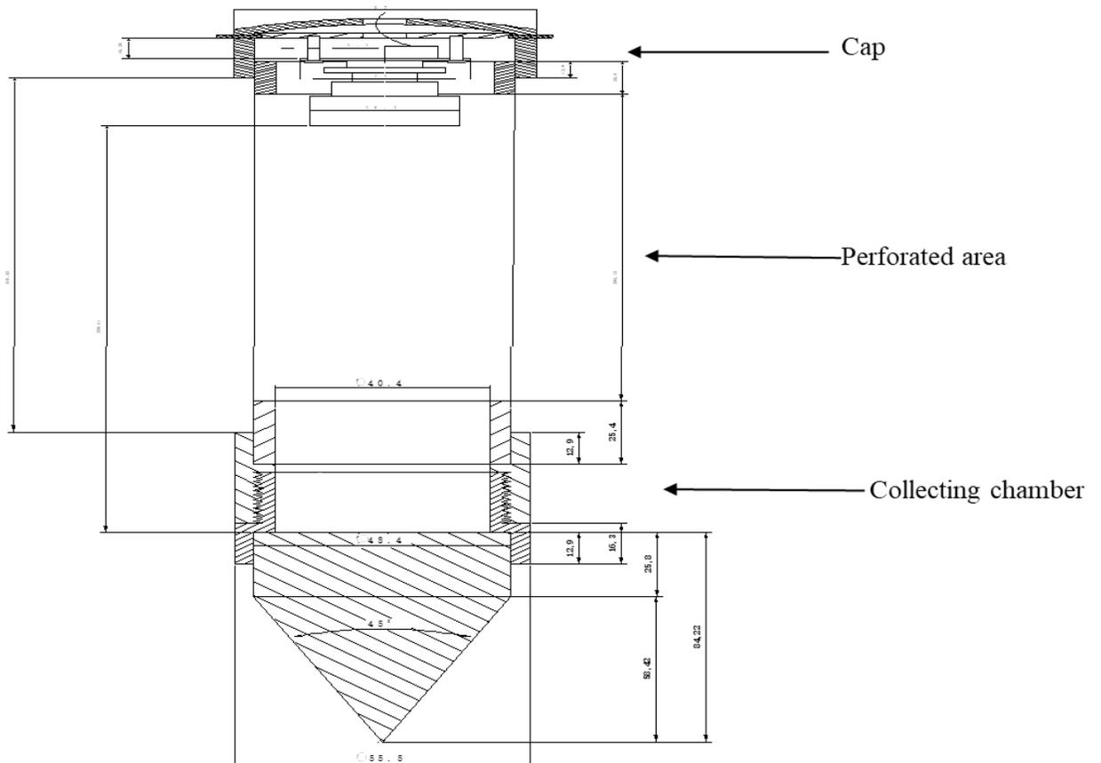
Fig.2. Schematic diagram for the insect trap. (Dimensions in mm)
