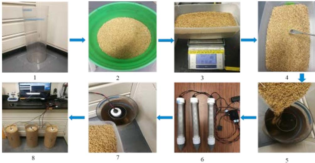
Fig. 9. Set up for lab test: (1) clear cylinder, (2) clean rice, (3) rice sampling, (4) sample infesting, (5) rice mixing, (6) developed traps, (7) trap assembling, (8) final set up.
