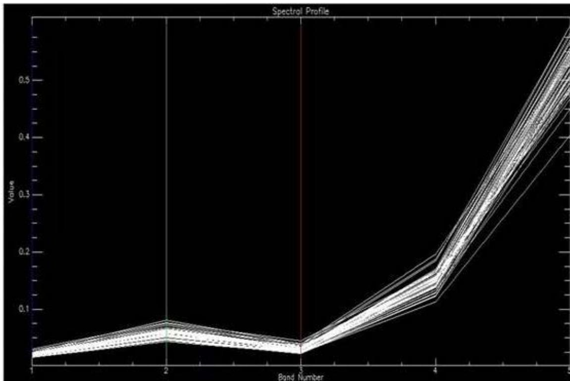
**Figure 5.** Spectral signatures of the 33 sample locations at the East Nicolaus site, plotted for the Micasense RedEdge's five wavelengths. No significant differences were found between the weedy rice, weeds (sprangletop, late and early watergrass), and M-206 rice variety.
