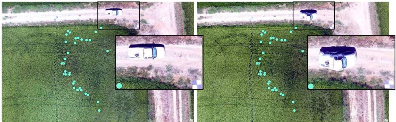
**Figure 4.** A 20mp red-green-blue (RGB) SODA 3D camera comparison from the East Nicolaus site. The nadir (straight downward) perspective is on the left and the oblique 90-degree south leaning perspective is on the right. Note: the truck highlights the angle perspective comparison.
