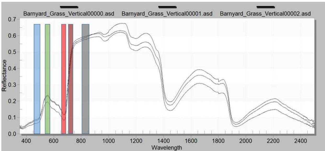
**Figure 2.** Comparison of the drone’s detection bandwidths versus the hyperspectral plots (from the barnyard grass data set). The bands indicate the Micasense RedEdge camera’s five spectral wavelengths (blue, green, red, red-edge, and near infrared).
