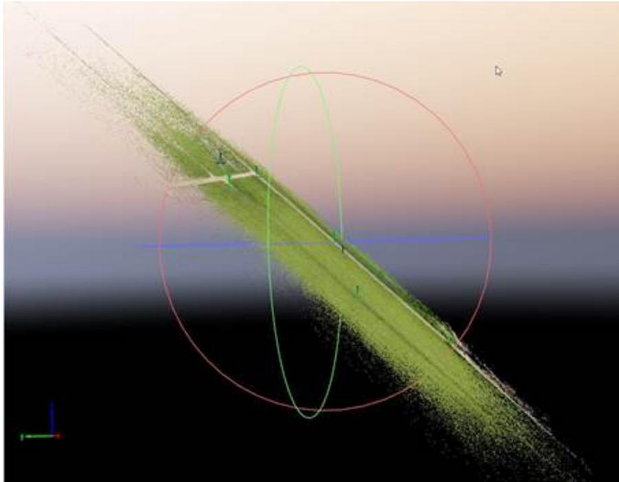
**Figure 3.** 90-degree 3D representation of the East Nicolaus red-green-blue (RGB) data. The blue line is the horizontal plane, green is east-west, and red is north-south. The 4 tiny anchor points are the adjusted ground control target (GCP) points.
