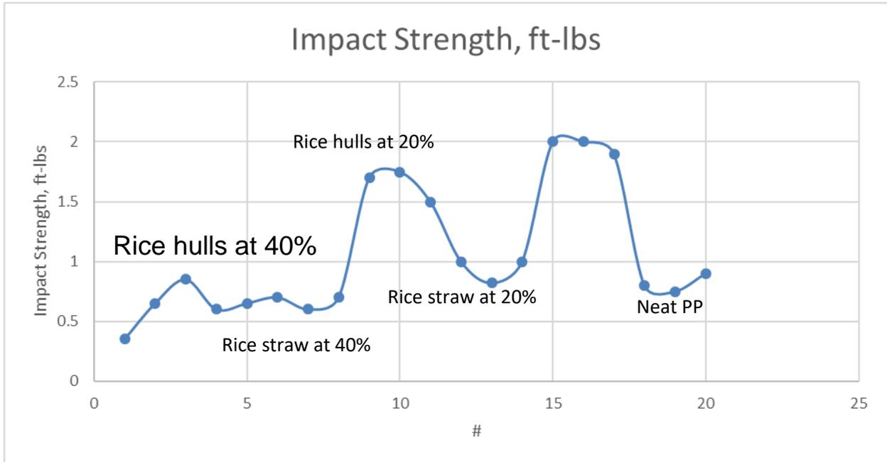
Figure 9. Izod impact test results for Rice straw and hulls.
