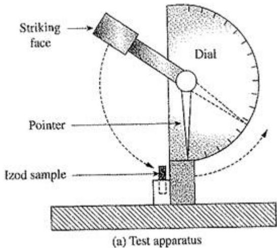
Figure 8. Izod impact test.
