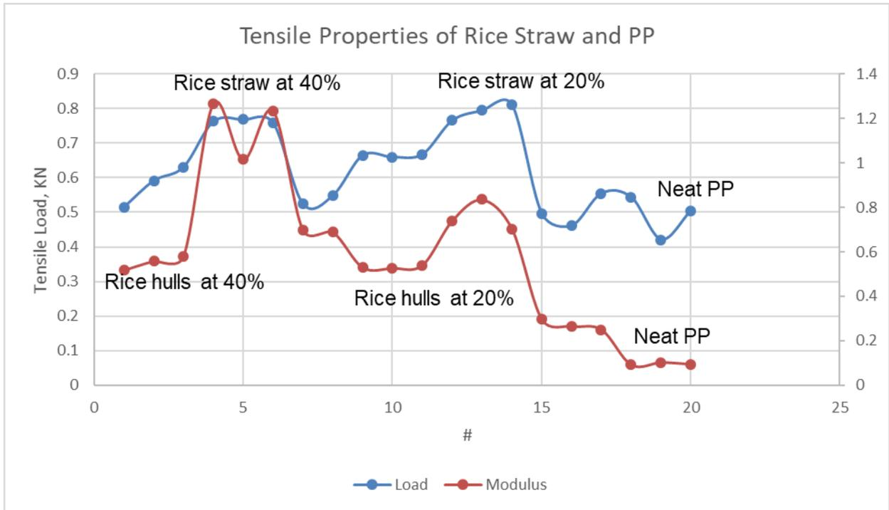
Figure 7. Tensile results for rice straw and hulls and PP.
