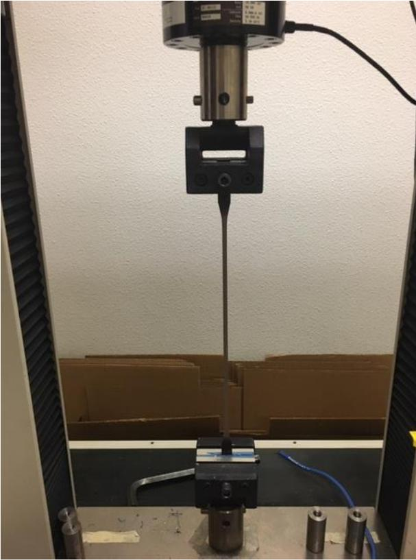
Figure 6. Tensile testing of PP and rice straw and hulls.
