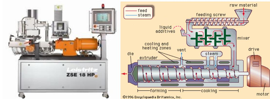
Figure 1. Leitztriz twin screw extruder with 40:1 L/D and 18 mm diameter.
