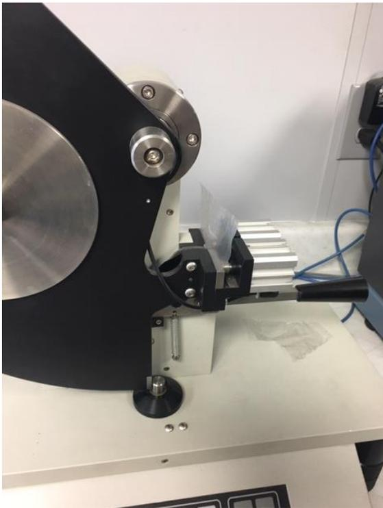
Figure 10. Tear strength tester
