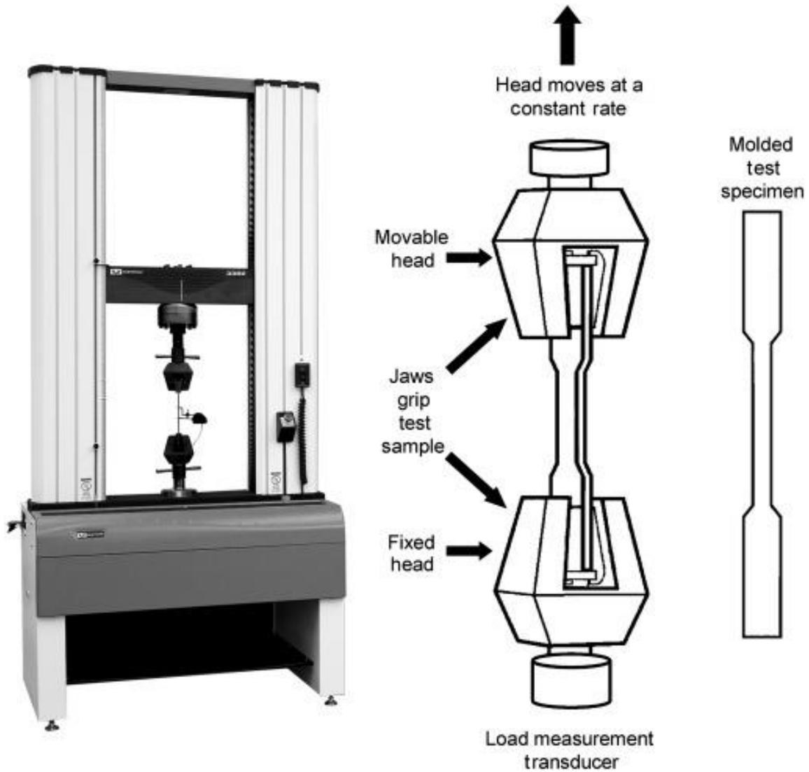
Figure 5. Tensile test machine.
