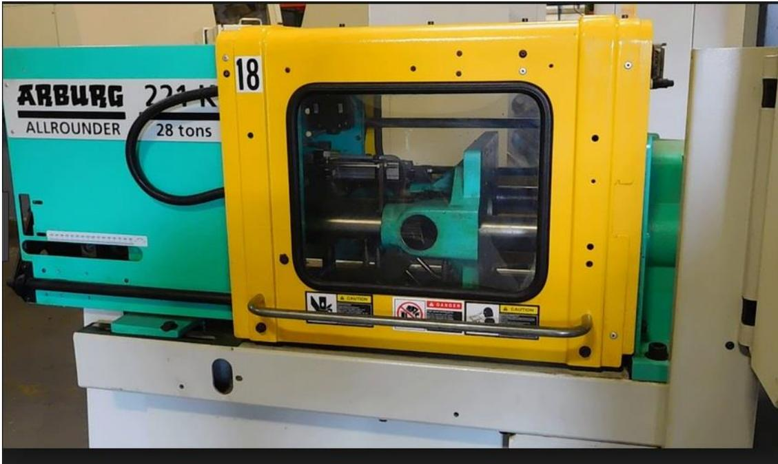
Figure 2. Arburg 28-ton injection molding machine.
