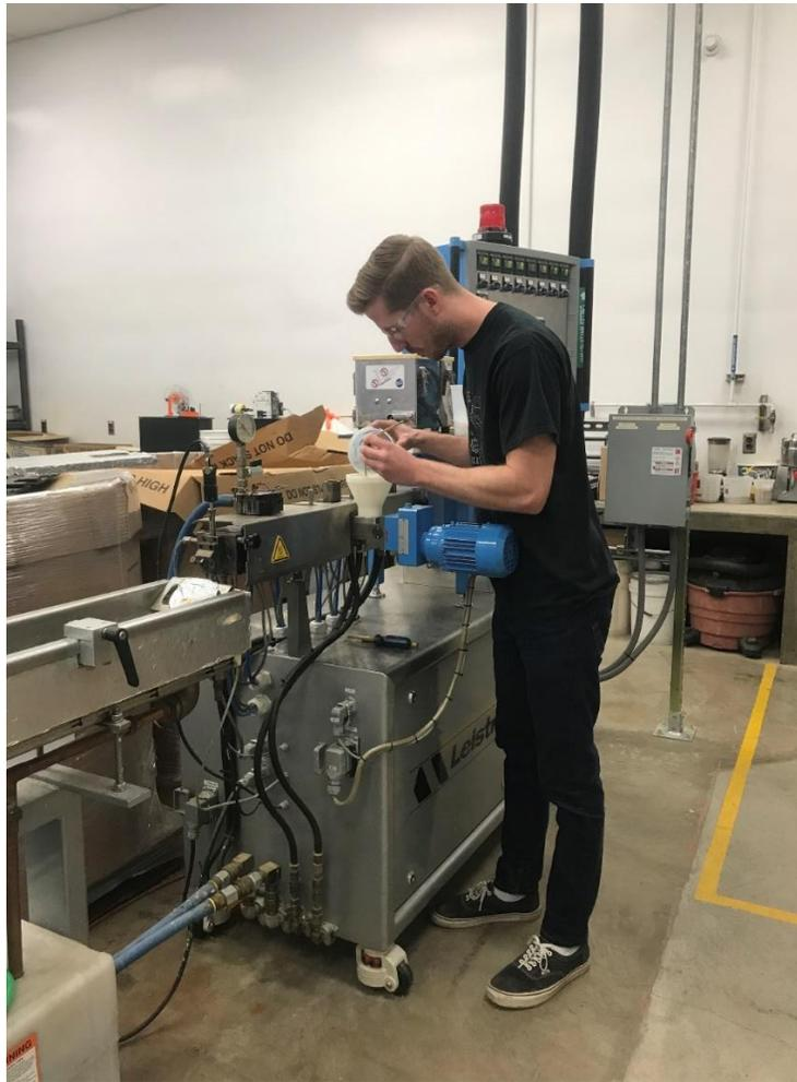
Figure 3. Student working on the twin screw machine adding rice straw and hulls.
