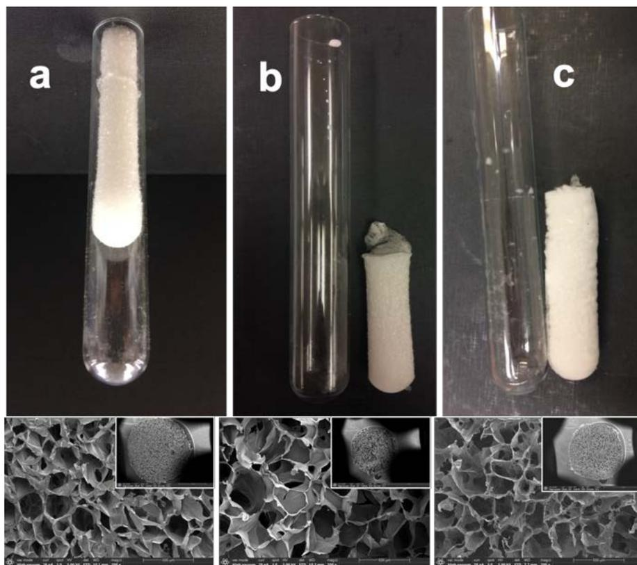
Figure 2. Aerogel shape retention as affected by protonation: (a) 11% (b) 46% (c) 100% COOH.
