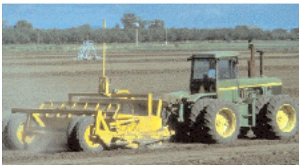
**Figure 2.** Typical scraper for leveling equipped with laser receiver that guides position of cutting blade. Signal is received from laser beam on stand in background.
